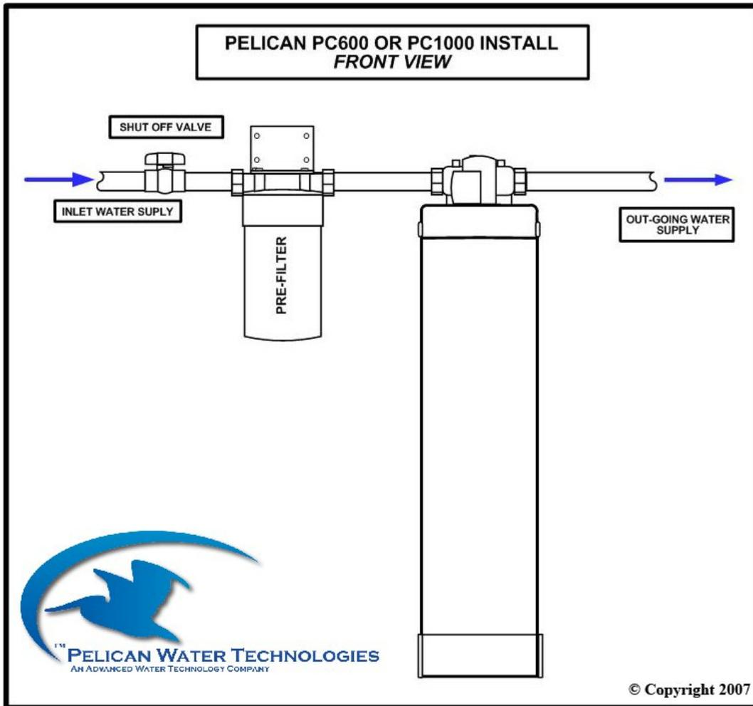
Install may vary depending on which side the main water supply is located.
