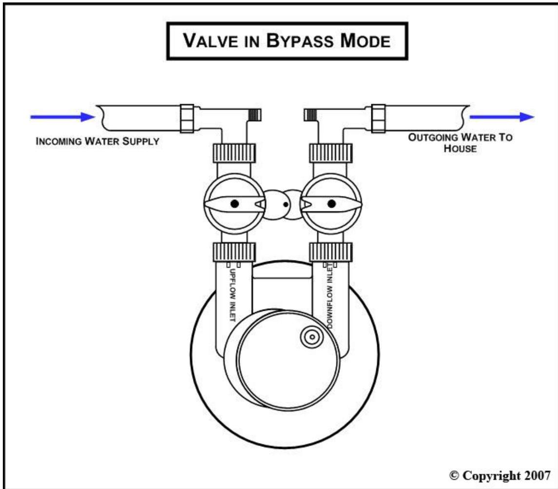
**Bypass Position:** Untreated water is supplied to the home. When the time comes to change the media this is the position to set the valve at.
