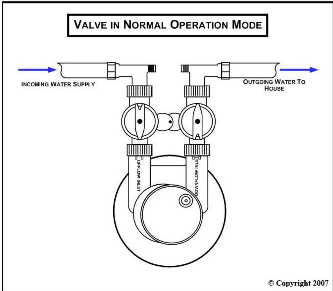
**Normal Operation Position:** Water flows through the control valve during normal operation.
